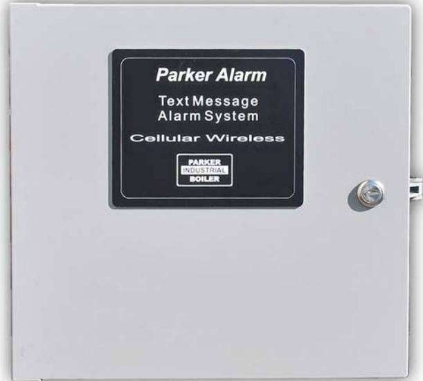
PV-A is standardly provided in a 12x12x4 plastic weather proofed Nema 1 enclosure to improve cellular transmission. It can be mounted indoors or outdoors and requires a 115V/60Hz/1Ph power source. It contains a UL Listed power supply and a Verizon Network certified cellular modem.
