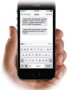
When an alarm condition is detected PV-A will text up to 3 phone numbers to indicate there is a problem. If the alarm is cleared an additional text is sent to let an offsite owner or operator to know.
