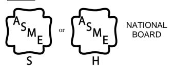
All Boilers are built in accordance with the A.S.M.E. Power & Heating Boiler Codes, Sections I & IV. Boilers above 15 PSI are furnished with the A.S.M.E. certification mark with an "S" designator and Trim. Boilers for 15 PSI are normally furnished with the A.S.M.E. certification mark with an "H" designator and Trim. All Boilers are inspected and registered with the National Board of Boiler and Pressure Vessel Inspectors.
